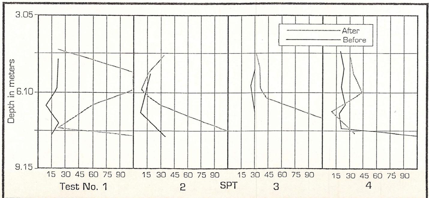
Fig. 4: Standard Penetration Test Results for After and Before Compaction Grouting
