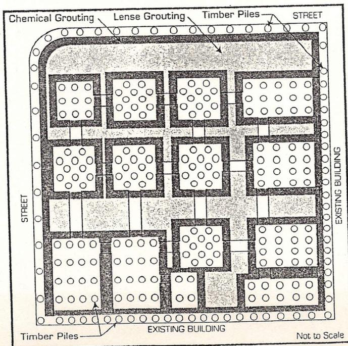
Fig. 6: Plan showing Chemical and Lense Grouting Zones
