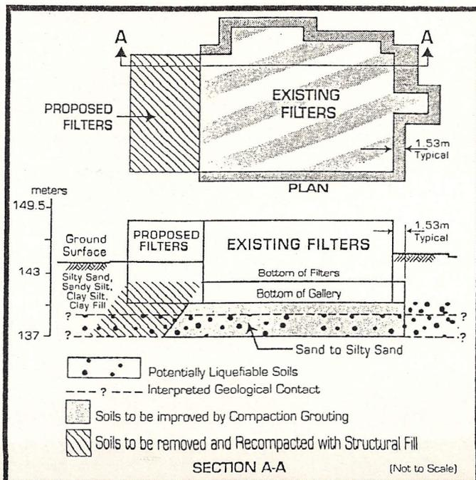
Fig. 2: Plan and Section of Areas Designated to be Densified using Compaction Grouting
