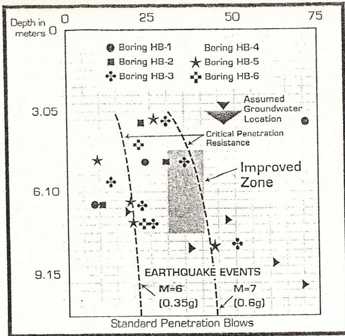
Fig. 5: Soil Improvement Relative to Earthquake Events
